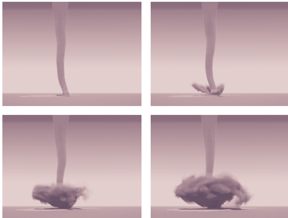
■ Figure A.7 Results from a large-eddy simulation showing the visual appearance of the debris and funnel cloud from a simulated medium swirl F3-F4 tornado. The funnel cloud is translating at 15 m/s and is ingesting 1-mm-diameter “sand” from the surface as it encounters a debris field. Please visit the book web site to access a full animation of this tornado simulation. (Photographs and animation courtesy of Dr. David Lewellen (Ref. 13) and Paul Lewellen, West Virginia University.)
