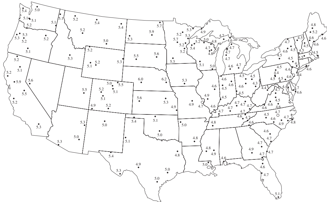
FIGURE 11 The pH of wet deposition shows that the worst acid rain occurs east of the Mississippi, where most of the coal-fired power plants are located. (Source: National Atmospheric Deposition Program; 2004 data from http://nadp.sws.uiuc.edu .)
