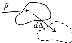
Figure 5.1 Force moving through a differential displacement.
