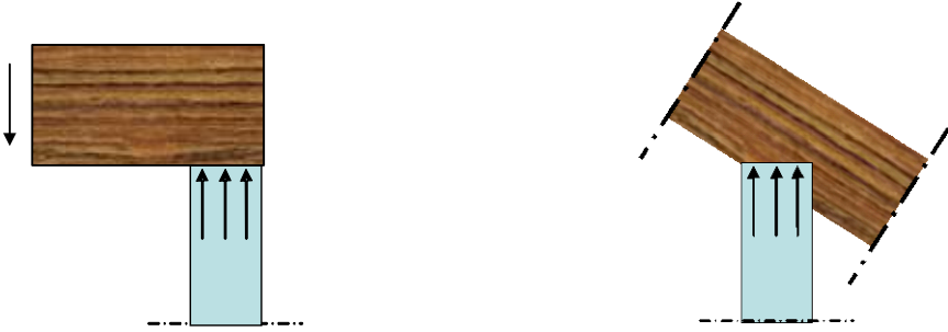
(a) Bearing perpendicular to grain. (b) Bearing at angle to grain. (Not covered.)
