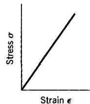
FIGURE 1.2 Linear stress–strain relation.
