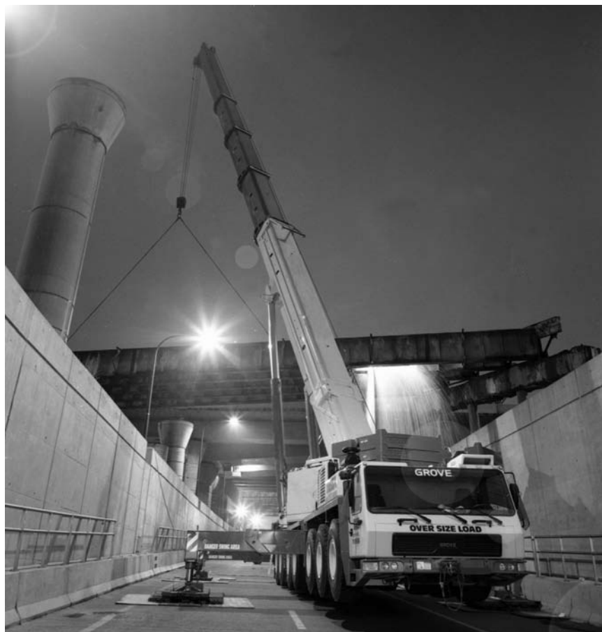
FIGURE 24. Large mobile hydraulic crane with telescoping boom. (Courtesy of Manitowoc)
