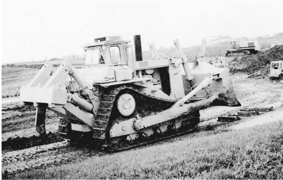
FIGURE 15. Heavy-duty crawler-mounted ripper. (Reprinted Courtesy of Caterpillar Inc.)
