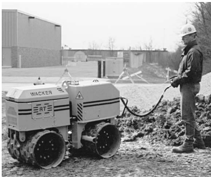
FIGURE 7. Walk-behind vibratory roller with remote control. (Courtesy of Wacker Corp.)
