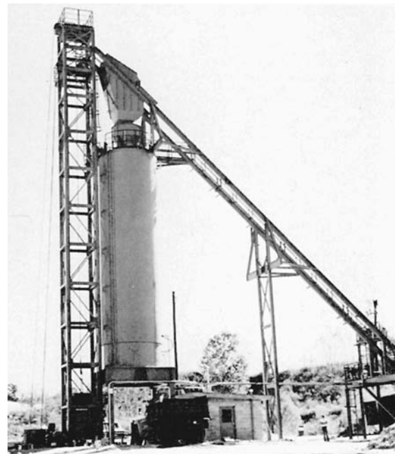
FIGURE 11. Insulated hot-mix asphalt storage bin with skip hoist. (Courtesy of Terex Road Building)
