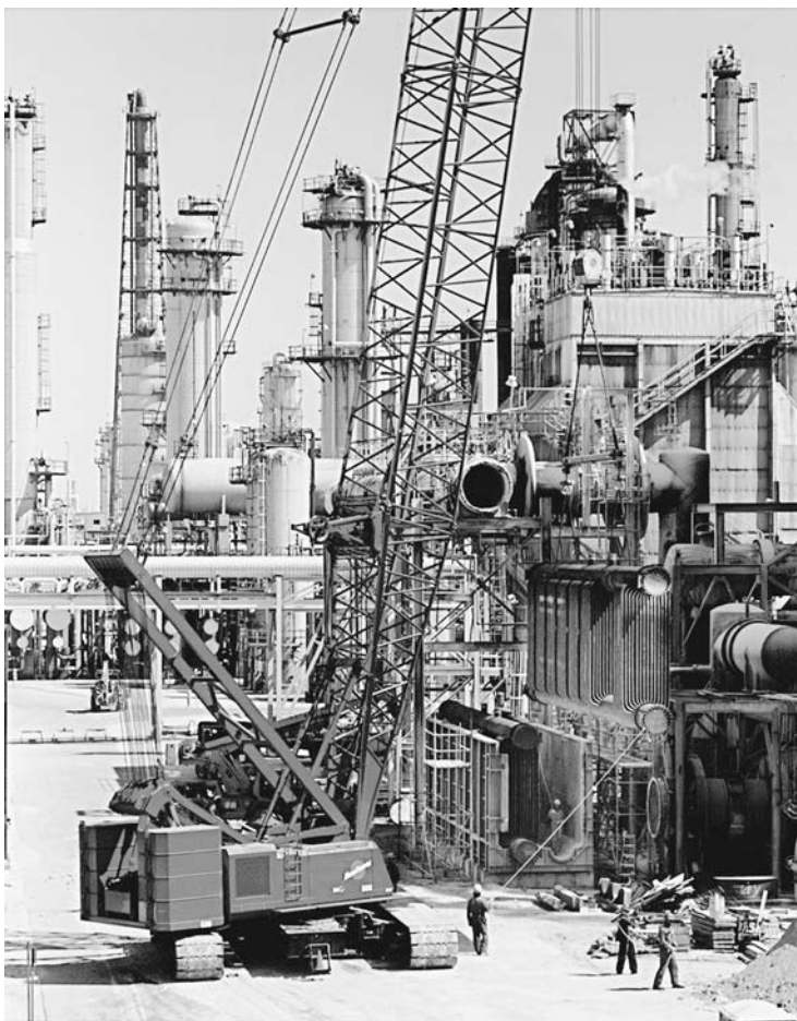
FIGURE 26. Large crawler-mounted lattice-boom mobile crane. (Courtesy of Manitowoc)
