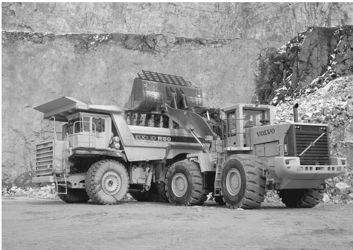
FIGURE 27. Forty-one-ton rear-dump truck. (Courtesy of Volvo Construction Equipment North America, Inc.)
