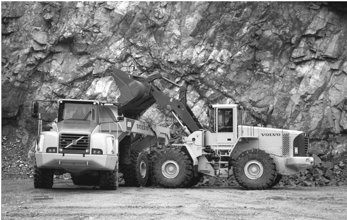
FIGURE 10. Articulated wheel loader with articulated hauler. (Courtesy of Volvo Construction Equipment North America, Inc.)
