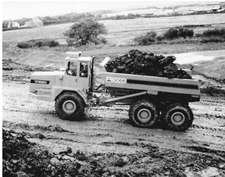
FIGURE 28. All-wheel-drive articulated dump truck. (Courtesy of CMI Terex Corporation)
