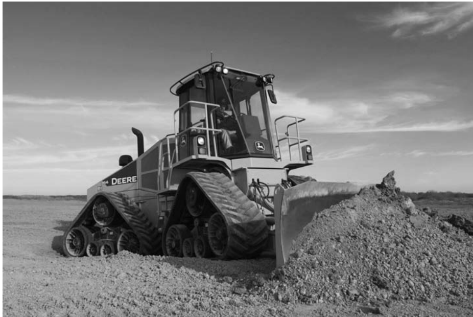
FIGURE 7. High-speed crawler dozer. (Courtesy of John Deere Construction & Forestry Company)
