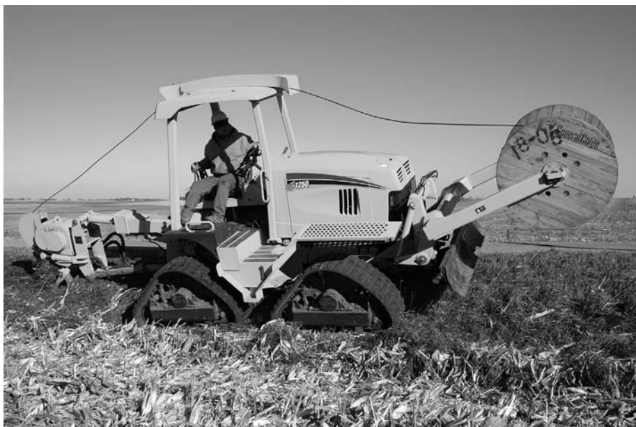
FIGURE 17. Hydrostatic vibratory plow. (Copyright © Vermeer Manufacturing Company, All Rights Reserved)
