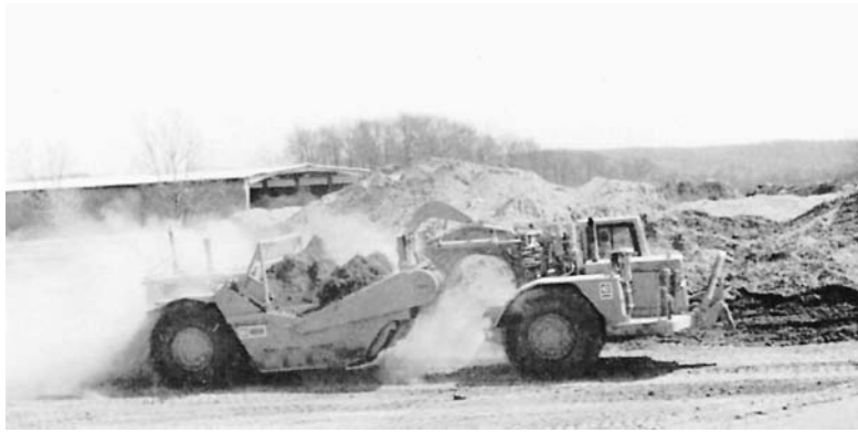
FIGURE 18. Twin-engine all-wheel drive scraper. (Reprinted Courtesy of Caterpillar Inc.)
