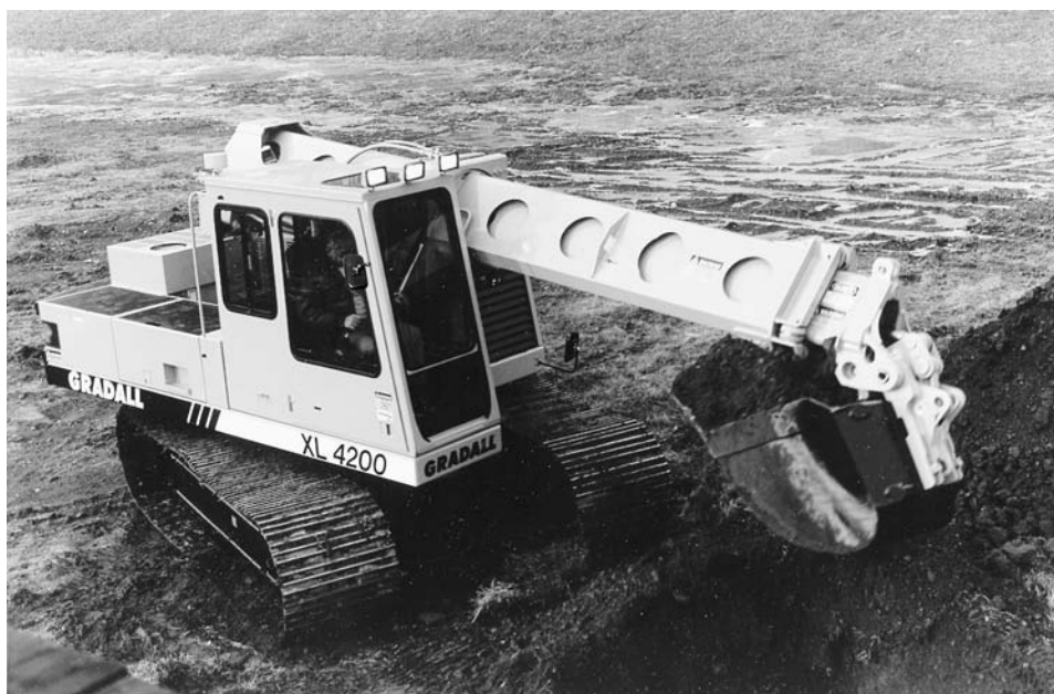
FIGURE 4. Telescoping-boom hydraulic excavator. (Courtesy of JLG Industries, Inc.)
