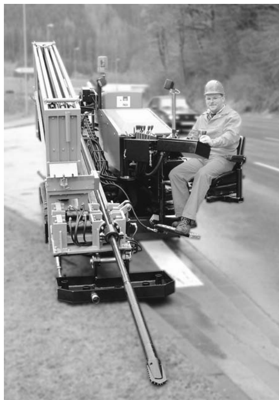
FIGURE 19. Thrust boring machine with percussive action. (Courtesy of TT Technologies, Inc.)
