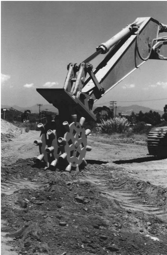
FIGURE 8. Compaction wheel mounted on hydraulic excavator. (Courtesy of American Compaction Equipment, Inc.)
