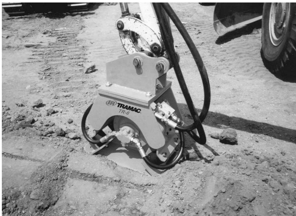
FIGURE 9. Vibratory plate compactor attachment for excavator. (Courtesy of Ingersoll-Rand Tramac)
