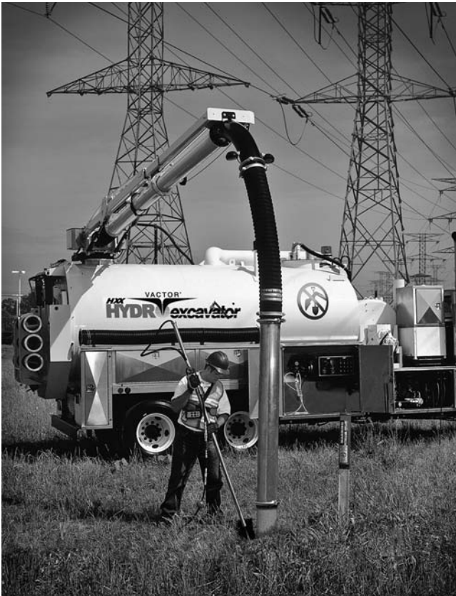
FIGURE 21. Vacuum excavator. (Photograph © Federal Signal Corporation. Used by permission. All rights reserved.)
