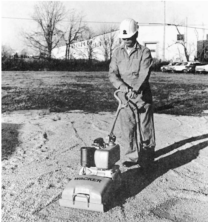
FIGURE 4. Walk-behind vibratory plate compactor. (Courtesy of Wacker Corp.)
