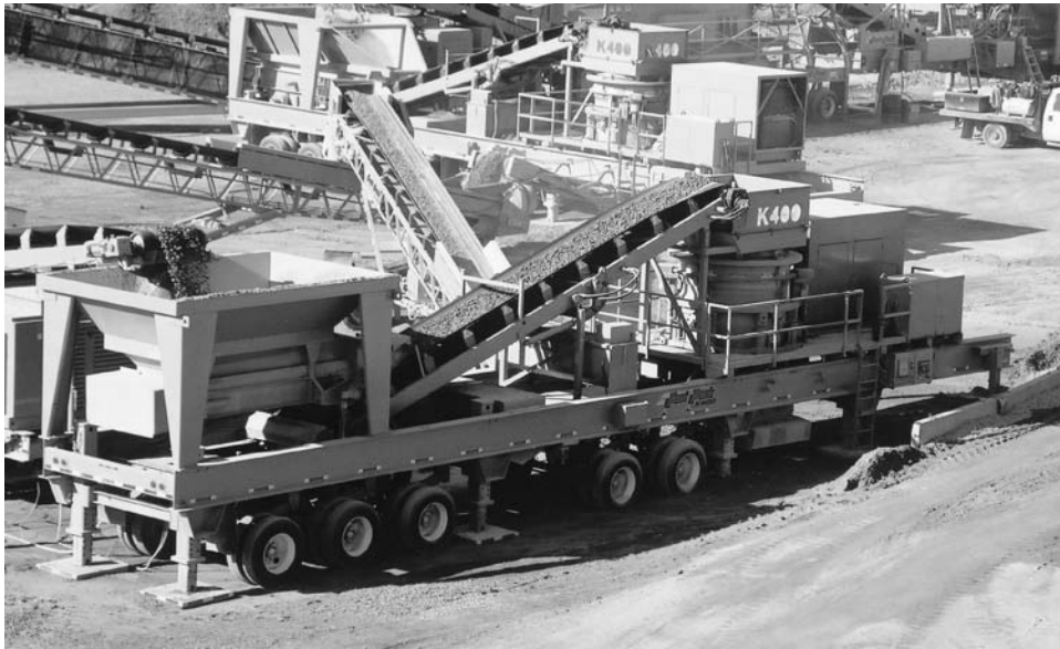
FIGURE 10. Portable recycled asphalt crushing plant. (Courtesy of Kolberg Pioneer, Inc., and Johnson Crushers International)
