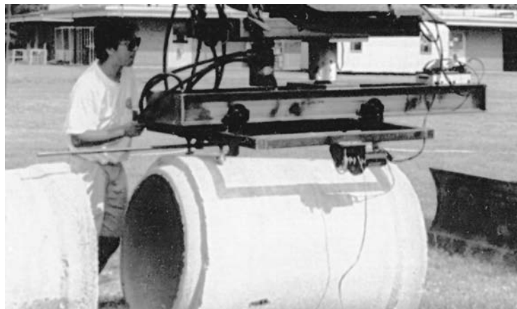
FIGURE 8. Remote-controlled pipe manipulator. (Courtesy of the Construction Automation and Robotics Laboratory, North Carolina State University)
