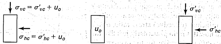
FIGURE 12.29 Conditions in specimen during a consolidated-undrained axial compression (CU) test.
