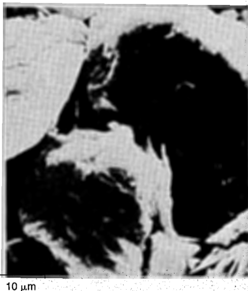
FIGURE 4.28 SEM of silt grain-to-grain contact in Swedish till (from McGown, 1973).
