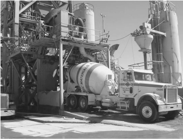
Figure 10-1 Centrally mixed concrete in a ready-mixed concrete plant. [Photograph courtesy of RMC Industries, San Francisco, CA.]
