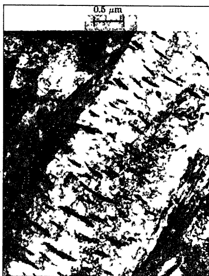
Figure 9.30 Precipitation of Fe_3C in Fe-0.39% C martensite tempered 1 h at 300°C. (Electron micrograph.)
