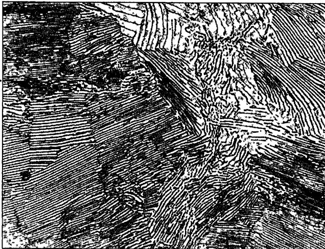
Figure 9.8 Microstructure of a slowly cooled eutectoid steel. The microstructure consists of lamellar eutectoid pearlite. The dark etched phase is cementite, and the white phase is ferrite. (Etch: picral; magnification 650 \times .) (United States Steel Corporation, as presented in "Metals Handbook," vol. 8, 8th ed., American Society for Metals, 1973, p. 188.)
