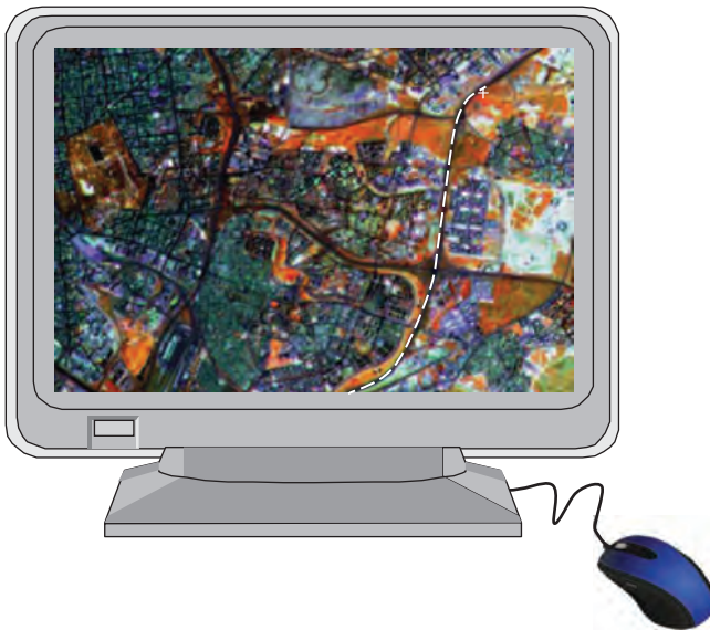
FIGURE 9.5 Satellite image used as a background source to update geographic information by manual digitizing.
