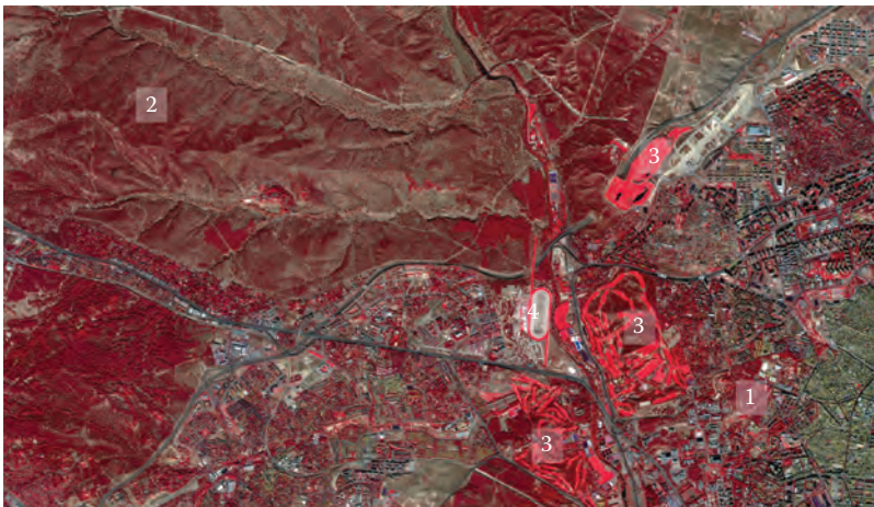
FIGURE 5.11 Spatial context and shapes in high-resolution images: (1) urban park, (2) natural forest, (3) golf courses, and (4) hippodrome. Fragment of the RapidEye image from the city of Madrid, Spain. (Image courtesy of BlackBridge, Berlin, Germany.)
