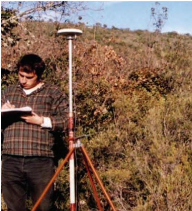
FIGURE 8.5 High-precision GPS receivers. These are important for ensuring a precise geometrical location in ground-truth surveys, particularly when working with high-spatial-resolution data.
