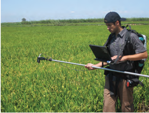
FIGURE 4.7 Spectroradiometric measurements in the field are useful in selecting the most useful sensor and spectral bands for a particular application. (Courtesy of M. Pilar Martin, SpecLab, CSIC, Madrid, Spain.)
