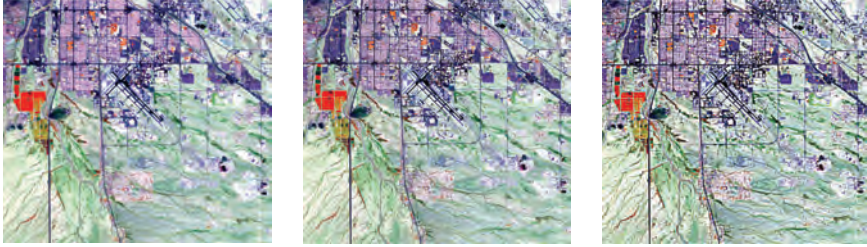
FIGURE 6.25 High-pass filters on a window of the Tucson OLI image. From left to right: original image, 3 × 3 filtered image, and 9 × 9 filtered image.
