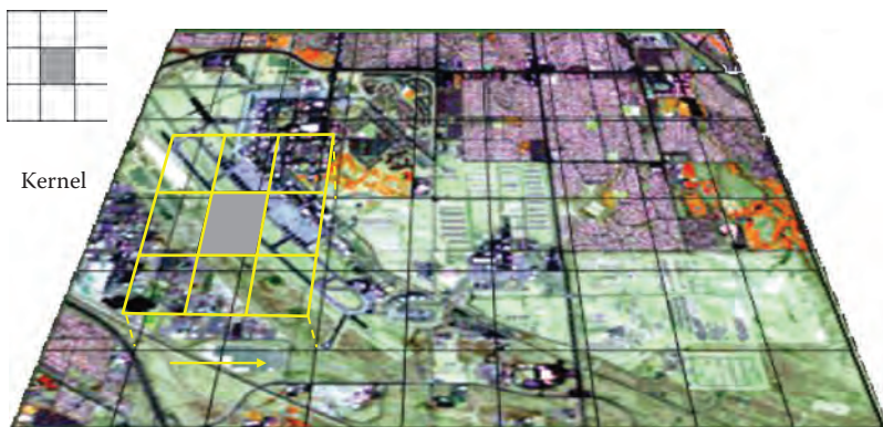
FIGURE 6.22 Filtering through the use of a spatial moving window (kernel) that is used to define the neighboring pixels.
