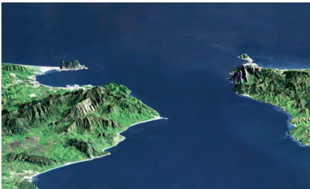
FIGURE 1.12 The Strait of Gibraltar in three dimensions, combining terrain data retrieved from the SRTM (see Chapter 3) mission with a pseudo-natural color image acquired by the Landsat TM in 1987. (From http://earthobservatory.nasa.gov/ )
