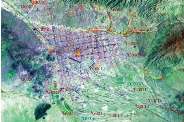
FIGURE 6.32 Ground control points selected to correct the Tucson image of 1986. Check points are displayed in blue.
