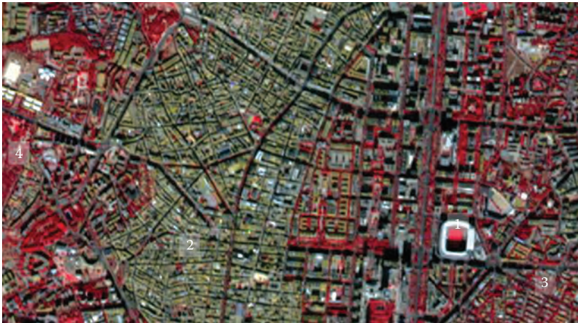
FIGURE 5.10 Textures on high-resolution images: (1) smooth, grass; (2) medium, concrete roof; (3) medium–high, gardened single-family housing; and (4) rough, trees. Fragment of the RapidEye image from the city of Madrid, Spain. (Image courtesy of BlackBridge, Berlin, Germany.)
