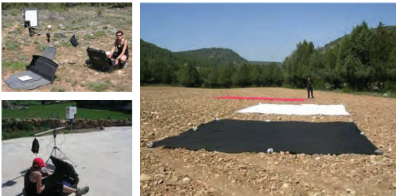
FIGURE 6.43 In situ measurements for atmospheric correction of an airborne campaign.
