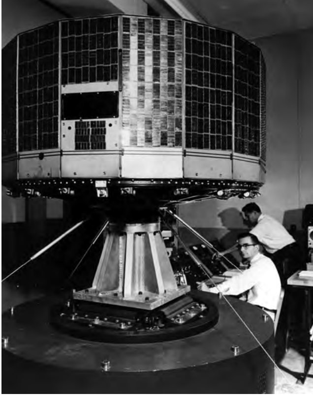
FIGURE 1.4 Scientist giving a vibration test to Television Infrared Observation Satellite (TIROS). The first TIROS was operational for 78 days. (From http://grin.hq.nasa.gov/ABSTRACTS/GPN-2003-00028.html .)
