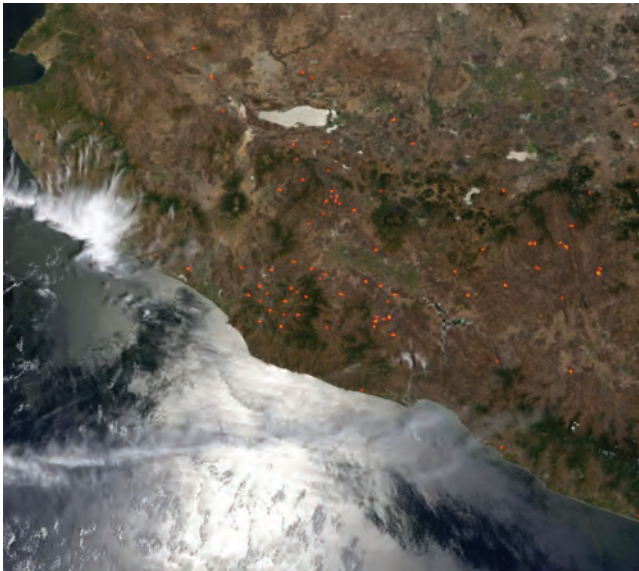
FIGURE 2.17 Terra-MODIS image of Mexico and Central America acquired April 13, 2004, showing Sun glint effects. Notice the white colors of Lake Chapala (central section of the image) and the Pacific Ocean to the south. (From http://visibleearth.nasa.gov/ )
