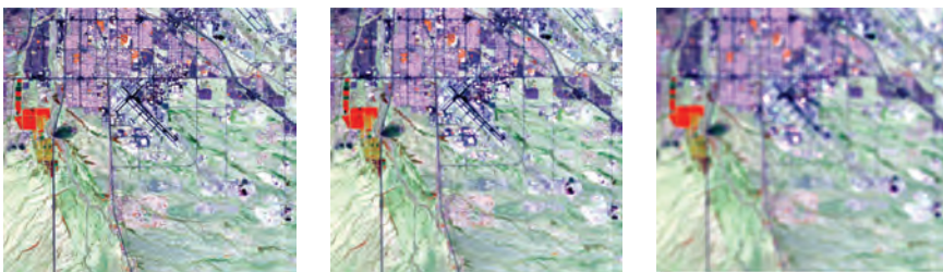
FIGURE 6.24 Low-pass filters of a window of the Tucson OLI image. From left to right: original image, 3 \times 3 filtered image, and 9 \times 9 filtered image.
