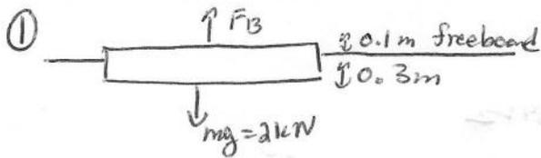
$$V_{\text{sub}} = 6\text{m} \times 7\text{m} \times 0.3\text{m} = 12.6\text{m}^3$$
