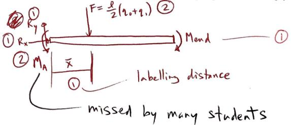
c. Solve for the external reaction loads (forces and/or moments) at A required to maintain static equilibrium of the beam. Clearly denote the directions of all loads. [8 points]
