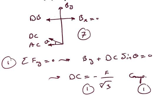
c. Using the method of joints, find the force in the truss member AC. Denote if the member is in compression or tension. [10 points]
