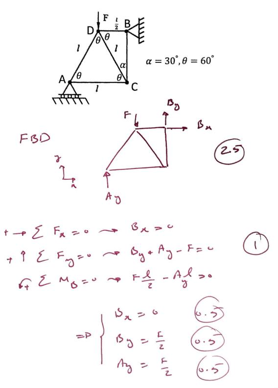
b. Using the method of sections, find the force in truss member DC. Denote if the member is in compression or tension. [10 points]
