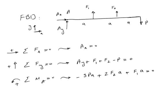
B) **[15 points]** Describe how you would solve for all the forces from part A. There is no need to solve the equations, but **write out any additional equations** that are needed and explain the principles and your logic. [Hint: number all of your independent equations, the total number of which needs to be the same as the number of unknowns].
