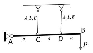
A) [10 points] Draw a fully labeled free body diagram of rod ACDB and write out the corresponding three equations of static equilibrium. Identify and label all unknown forces.
