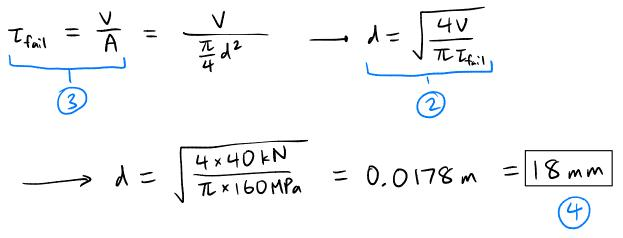
C. **[4 points]** What would be the minimum required bolt diameter if the design specifications required a factor of safety of 3.0?
