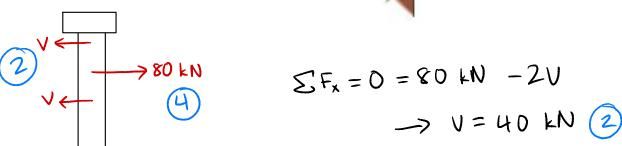
B. **[9 point]** Determine the minimum required bolt diameter (to the nearest millimeter) so that it will not fail in shear under the loading shown.
