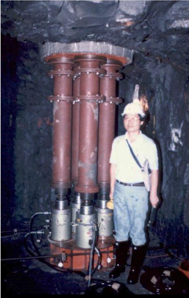
Figure 7: A plate loading test to determine the in situ deformation modulus of the rock mass exposed in an exploration adit.
