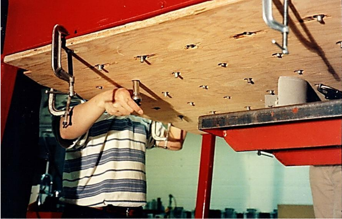
Figure 12: Holding the bottom nut during bolt tightening.
