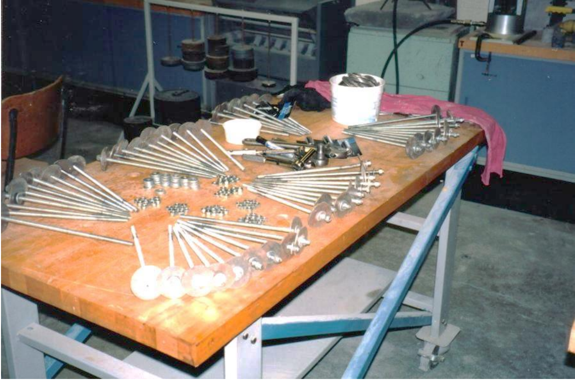
Figure 4: Miniature rockbolts ready for installation.
