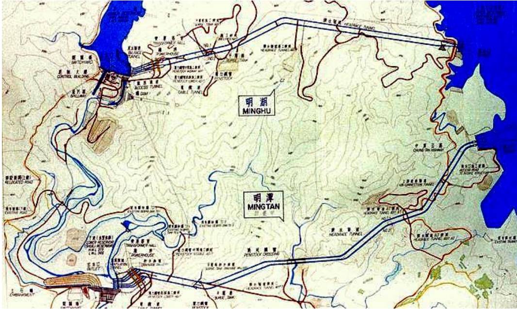
Figure 2: Plan showing the layout of the Minghu Pumped Storage Project (top) and Mingtan Pumped Storage Project (bottom).
