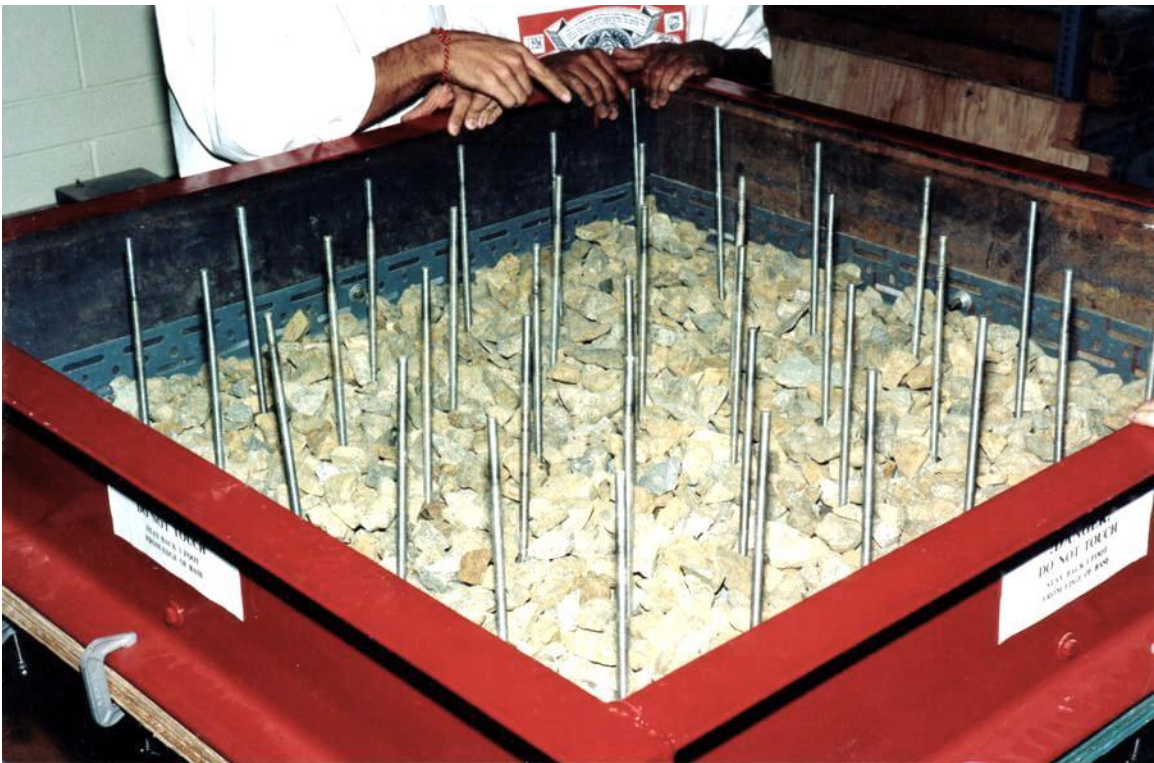
Figure 9: Placing the gravel in the frame.
